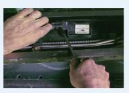
**4.** Remove two bolts to release the sensor.
