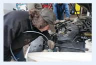
3. Pump out the windshield washer fluid.
