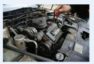
2. Pump out the power steering fluid. This hand pump can also be used for other oils.
