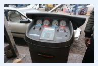
**3.** The certified refrigant technicial must record the amount of refrigerant removed from each vehicle.
