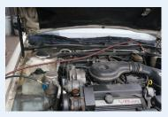
2. Start the refrigerant removal machine and remove all Freon gas from the vehicle.
