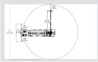
Do not site baler under power lines, communication lines, etc. The grapple extends 35 ft vertically
